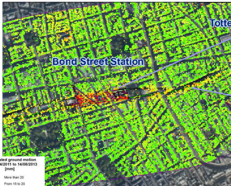
Accumulated ground motion from 28/04/2011 to 14/08/2013 [mm]
