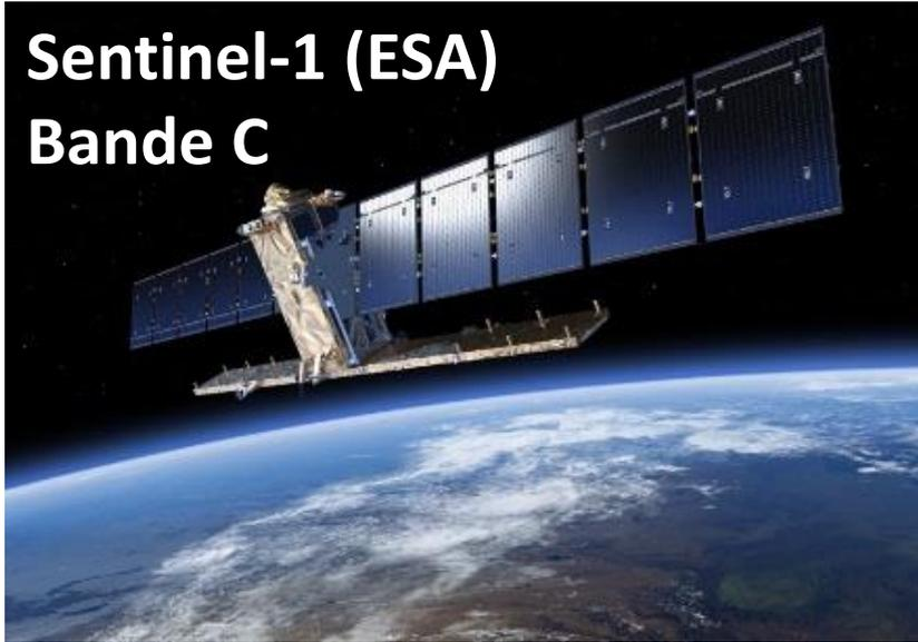
mode TOPSAR. 250km swath width; 5m-x-20m ground resolution.
